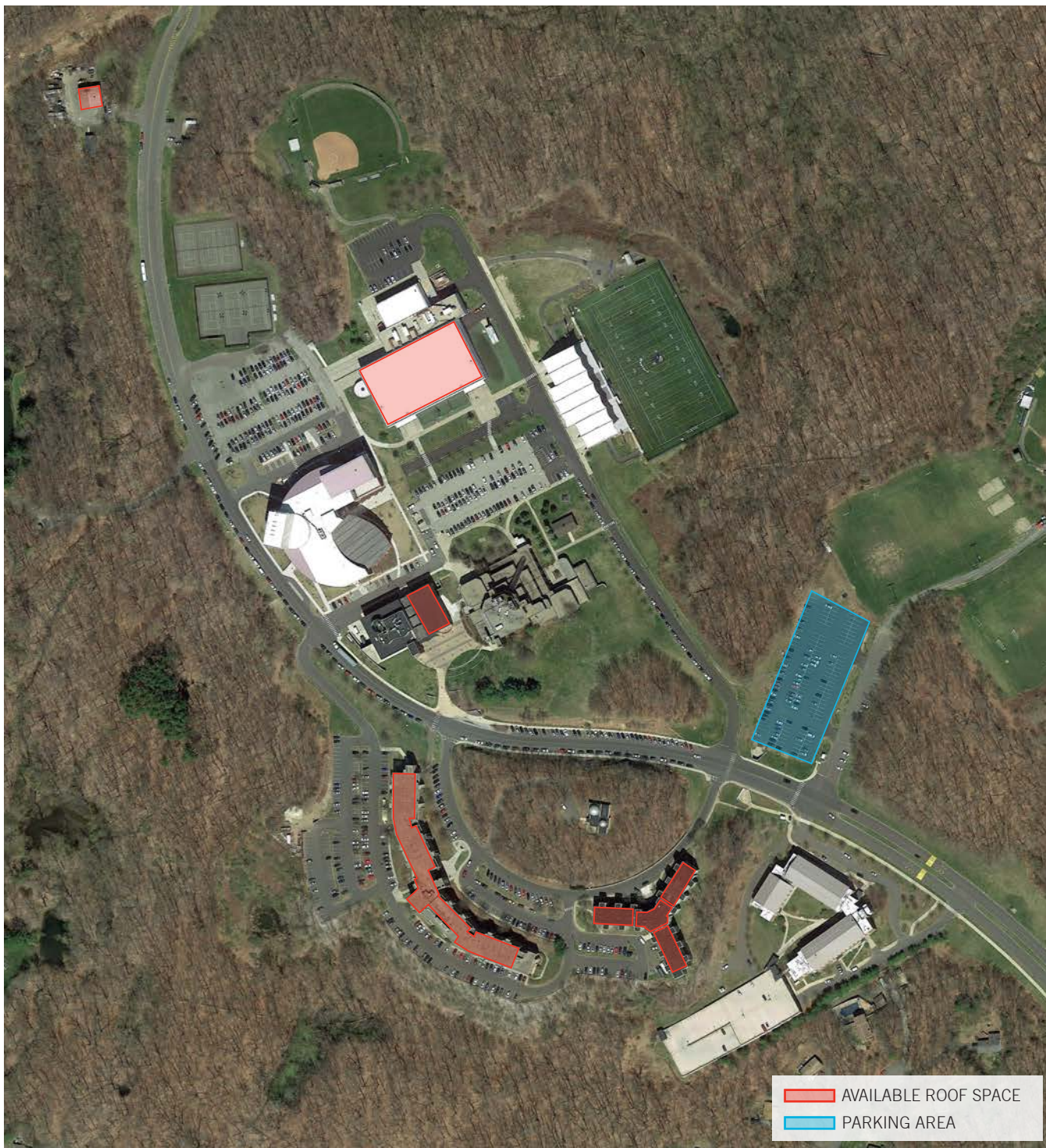
FIGURE 2.7: Western Westside Campus Potential Areas for Solar PV
