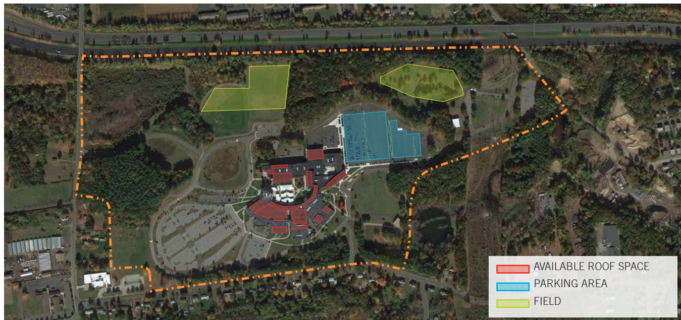
FIGURE 2.7: Manchester Campus PV Potential
