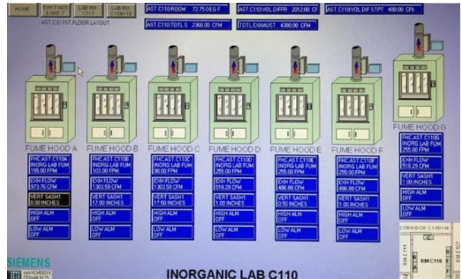
FIGURE 2.5: Manchester BMS - Fume Hoods
