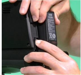
Start by putting on the battery. Look at the battery and locate the electrical connectors. These will go in first. Slide the battery in and push until you hear a click. It may take a few tries. To take the battery off push the gray button next to the battery and pull the battery out.
