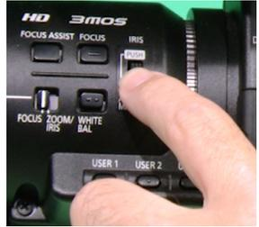
You will want to use the camera in manual mode so that your exposure, focus and color balance are correct. Not all cameras are good in auto. First make sure the switch is in manual. Next look in the view finder and you will either see a number in DB or AGC. If it is in AGC push the iris wheel in to change the setting. Once you have the iris in manual where you see a number you can now move the wheel up and down to open and close the iris to get the correct exposure.
