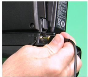
Next make sure the line/mic switch is set to mic because that is what we are using. Now plug in the male side of the xlr into channel one. To remove the xlr, push in the tab above the connector and pull the xlr out. You will want to use headphones to monitor the audio. Take the headphone connector and plug it into the headphone jack located just under the battery release button.
