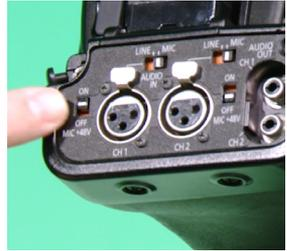
To plug in the xlr into the mic and the camera make sure to line up the pins with the cable. Push in the cable and make sure it is tight. To remove the cable push in the button on the cable pull on the connect and the microphone to separate the two. On the back of the camera there is a switch to provide 48 volts to the microphone. Depending on the type of microphone you are using you may or may not need this switch on.
