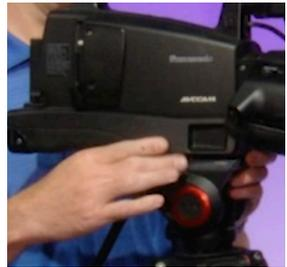
If it is not balanced the camera will fall to one side or the other. If it is not balanced loosen up the plate screw and carefully slide the plate to make the camera balanced. Tighten up the plate screw and recheck. You may have to do this a few times.
