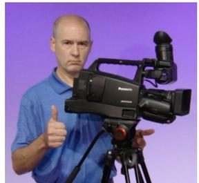
You know you are well balanced when you let go and the camera doesn't fall front or back. Most importantly never leave the tripod without locking the tilt and pan knobs. Otherwise the camera will fall, and you could possibly damage the camera and/or tripod.
