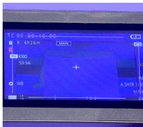
Once you are on Ach or Bch place a white card in your shot where you will be shooting. Zoom in so that the white card fills as much as possible of the frame. You may have to open or close the iris a bit to get a proper exposure. Now press and hold the white balance button until LCD screen goes black. You will then see a confirmation window saying WB set ok. Make sure to reframe your shot and fix your iris if needed.
