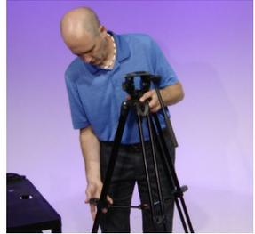
Take the tripod and unscrew the arm and extend it out and way from the legs. While holding the tripod like a baby, unlock and extend the lower legs. Extend the legs and place the tripod on the ground. Be sure to push down the center support so that the legs are secure. Depending on what you will be shooting you may have to raise or lower the tripod to get the correct shot.
