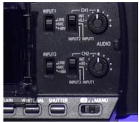
Depending on which input you are using switch to mic. Depending on the type of microphone you are using you may or may not need 48 volts. In this example with our hand-held mics we just need mic. On channel two, make sure that you select input two.
