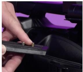
To put the camera plate on the camera, locate the front of the plate indicated by an arrow showing where the lens should be placed the brass pin in the front hole on the bottom of the camera. Screw the bolt in the second hole. Use a coin or the side of a key to make sure the bolt is tightened. Make sure the lock is loose and slide the camera plate on from the back to the front while holding the red pin in. Once the plate is on and in the location you think you want tighten up the lock.
