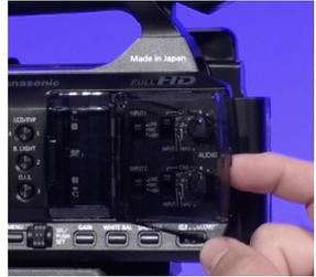
To plug in the XLR into the mic and the camera make sure to line up the pins with the cable. Push in the cable and make sure it is tight. To remove the cable push in the button on the cable pull on the connect and the microphone to separate the two. On the side of the camera there is a clear door. Gently pull the door open from the right side.
