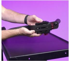
If you use the AG AC30 camera you will notice that the camera is half the size of the other cameras we use. If you plan to shoot on a shoulder you will need a shoulder rig to help you keep your camera shot stable. First loosen the lock slide of the plate back while pressing the red pin in. If you don't press the red pin in the plate it will not slide out.
