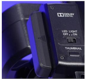
On the side of the camera is a small door in the middle of the camera is where the SD card will go. Gently pull the door from the left side to access the SD card slots. Take your SD card and slide it in slot number 1 with the brass contacts facing the front of the camera. Push it in then close the door. On the top front left of the handle you will see lines that will make up an arrow.
