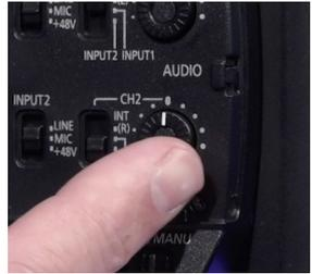
Now make sure you are in manual for audio level control. Press the menu button. Scroll until you see Audio setup and press select. Audio level ch1 and ch2 should be in manual. If not scroll to that channel and press select. Scroll to manual and press select. Scroll to exit and press select. While using the audio dial for channel two, which is your external microphone, you can adjust the level.
