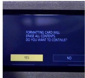
Press menu and scroll to Other Function. Format should be already highlighted. Press select. Pick which SD card slot you would like to format. Word of caution make sure you have removed your footage before you continue. Scroll to the SD card and press select. Scroll to highlight yes and press enter. You will be asked again, do you want to continue, scroll and select yes. Once done press select to exit.
