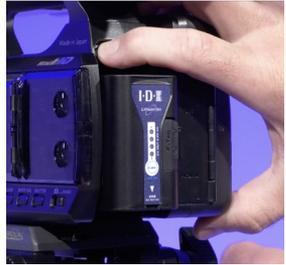
Start by putting on the battery. Look at the battery and locate the electrical connectors. These will go in first. Slide the battery in and push until you hear a click. It may take a few tries. To take the battery off push the button on the top left of the battery compartment and slide the battery up and pull the battery out.
