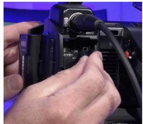
Now plug in the male side of the XLR into channel two. Make sure the connector is all the way in. To remove the XLR, push in the tab above the connector and pull the XLR out. You will want to use headphones to monitor the audio. Take the headphone connector and plug it into the headphone jack located on the right side of the camera under the audio 2 input. Gently lift up the door where the headphone symbol is.
