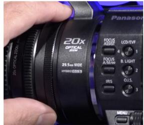
Once you have the iris in manual where you see F and a number or open, you can now move the iris ring which is the ring closest to the camera body up and down to open and close the iris to get the correct exposure.
