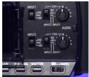
Looking in the LCD you will see a bar and dots on the bottom of the viewfinder. This shows you the audio level for each of your channels. First look at channel two and adjust the level using the dial. Adjust the level so that the audio is peaking just past the vertical line which indicates good audio levels.
