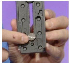
On the top there will be a screw on the right side, this will unlock the plate from the tripod. On this tripod loosen up the screw and push it down and lift the plate out. On some tripods there will be a button either on the back or side that you push and slide the plate off. On the bottom of the plate you will see an arrow showing which side the camera lens needs to be. Make sure you have this side of the plate near the lens.
