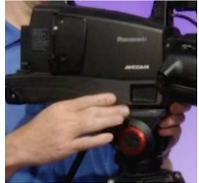
If it is not balanced the camera will fall to one side or the other. If it is not balanced loosen up the plate screw and carefully slide the plate to make the camera balanced. Tighten up the plate screw and recheck. You may have to do this a few times.
