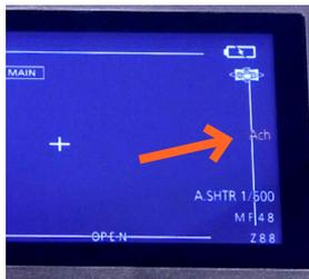
Always do a manual white balance. While looking at the LCD push the white balance button to get out of ATW. Once you see something other than ATW use the scroll wheel and look for either Ach or Bch.
