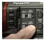
In this case we are plugging into channel 2. To adjust audio settings look on the side of the camera with all the buttons, there is a clear door. Gently pull the door open from the right side. Depending on which input you are using switch to mic. In our case we pick channel 2. Depending on the type of microphone you are using you may or may not need 48 volts, better known as phantom power. In this example with our hand-held mics we just need mic.
