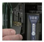
On the rear left side of the camera is a door where the SD card will go. Gently pull the door from the right side to access the SD card slots. To take the sd card out gently push on the sd card. The card will pop out a bit so you can grab it. To put it back in take the SD card and slide it in slot number 1 with the brass contacts facing the battery. Push it in then close the door.
