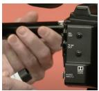
To plug in the xlr into the mic and the camera make sure to line up the pins with the cable. Push in the cable and make sure it is tight.
