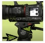
While holding the camera from the handle, slide the camera and plate on to the tripod head from the back. Before you tighten up the plate you will want to balance the camera on the tripod head. While holding the camera, loosen up the tilt nob and see if the camera is balanced on the tripod. You will want to redo the balance when you add items to your camera like a battery, cables, monitor ect. Most importantly never leave the tripod without locking the tilt and pan knobs.
