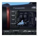
Finally, the side with all the buttons, switches, and rings. First let's look at the lens. There are three rings. You have the focus ring, zoom ring and iris. On the body of the camera is the ND filter (for use outside in bright light), iris, focus assist, Focus auto/manual and focus auto button. Just past the red ring you have O.I.S (optical image stabilization), zebra, WFM (Waveform Monitor), A.iris level (Auto iris).
