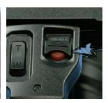
On the side with the handle grip, you have power and the record button. On the top is the zoom control, rec check and iris. Behind the handle grip are various connectors. You have SDI out, TC or Timecode in/out, and audio input 2. On the top handle is another record button that has a protective cover so not to trigger the recording on/off by accident. To access the record button, slide the cover to access the button. Next to that is another zoom control.
