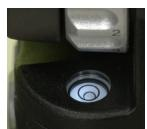
On the head of the tripod there will be a bubble level to help make sure that your tripod and camera are level. Our tripod also has a light on it. The button to turn it on is located on the side of the bubble level. Loosen the screw under the head and the head will be able to be moved around. Move the head so that the bubble level is in the center of the circle.
