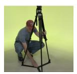
To open and set up the tripod hold the tripod like a baby, unlock and extend the lower legs. Extend the legs, lock the screws, and place the tripod on the ground. Be sure to push down the center support so that the legs are secure. You can extend the spreaders to widen the base.
