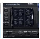
Next to that behind the cover are the audio controls. Very important is the headphone jack located just above the 4k logo behind the rubber cover. On the bottom you have gain (which is 0, 6 and 12db), white balance, shutter, menu, scroll/select wheel, exit, display/mode check (turns on/off the display you see on the screen), auto/manual, and slot sel (pick which SD slot you want to use if you have 2 sd cards in).
